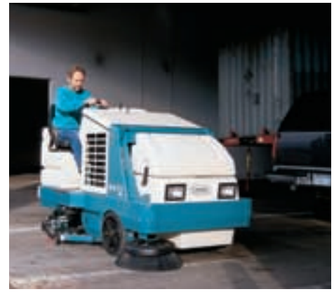
The 8210 automates both sweeping and scrubbing to make operators more productive.
