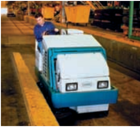
The 8210's scrub head extends to clean tight against edges, pallets and machinery. Optional on the 8200.
