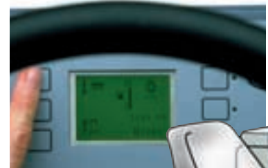
The 8210 has an intelligent, LCD control panel that tells the operator when to perform maintenance, uses audible reminders and even diagnoses problems - in 12 languages!
